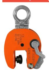
For vertical lifting and transporting (thin) sheet metal. Special movable pivot in the clamp provide extra pressure on the material, eliminating the risk of slippage.
